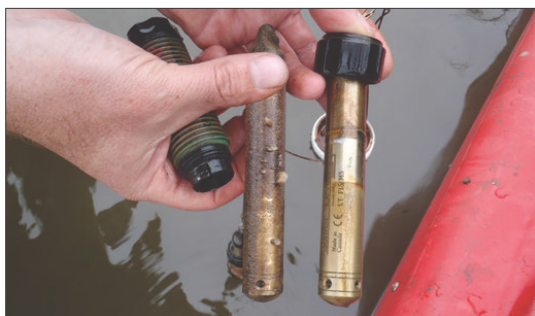
The Levellogger on the right was protected using a Biofoul Screen, while the Levellogger on the left was deployed unprotected and shows signs of biofouling on the sensor end.
