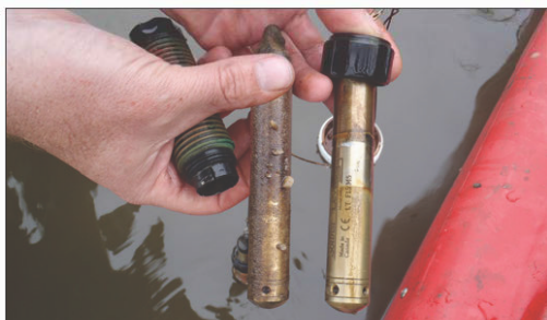
The Levelogger on the right was protected using a Biofoul Screen, while the Levelogger on the left was deployed unprotected and shows signs of biofouling on the sensor end.
