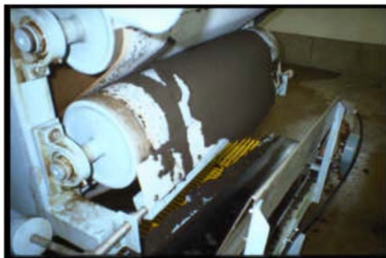
FIGURE 2 DEWATERED SOLIDS CAKE DROPPING FROM BELT FILTER PRESS AFTER PROCESSING
