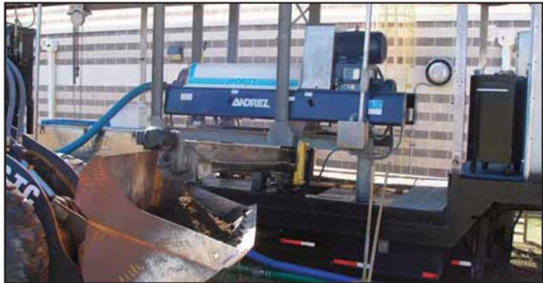
Centrifuge pilot unit
