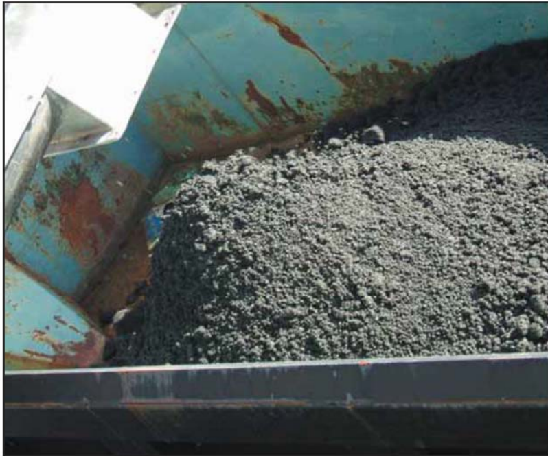
Dewatered sludge cake from South Water Reclamation Facility
