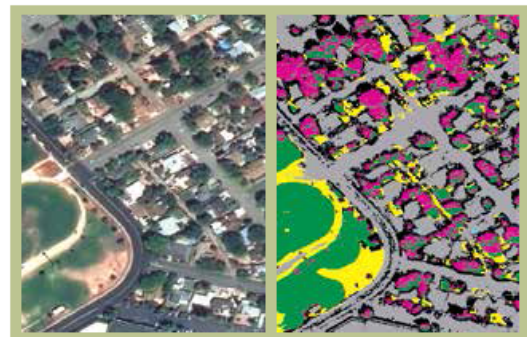
OmniEarth analyzes satellite and aerial imagery to automatically classify land use by cover types, such as grass, trees or man-made surfaces.
