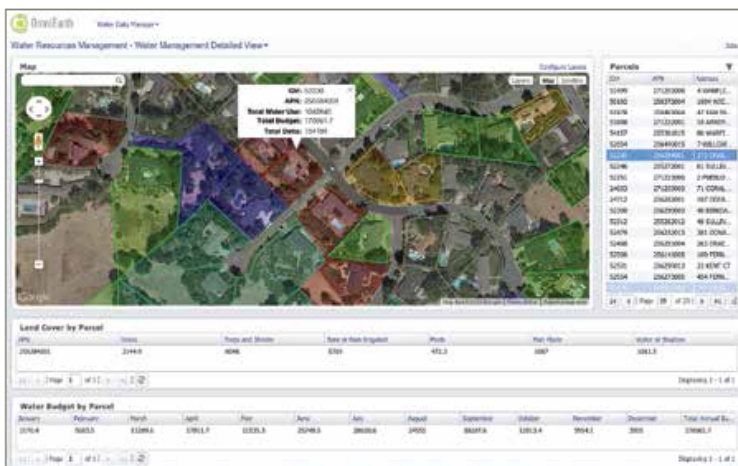
OmniEarth's cloud-based solution combines satellite and aerial imagery, parcel boundaries and water meter data to help water resource managers maximize conservation outreach.
