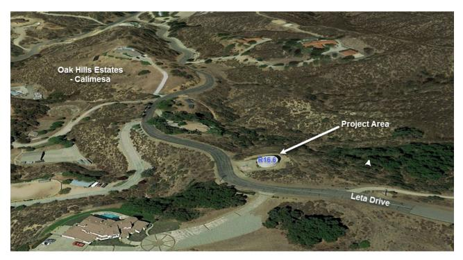
The project will consist of removal of the existing drinking water reservoir (bolted steel tank) and installing a new tank within the same location and footprint. The existing tank has a diameter of 38 feet, with a height of 24 feet. The replacement tank will measure 47 feet in diameter, 32 feet tall. The center point of the new tank will align with the existing tank, increasing the circumference by 4.5 feet. See the figure below.
