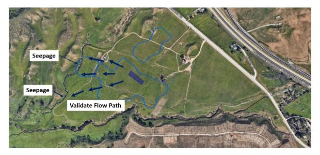
The following illustration shows how it is possible for the recharge water to move laterally instead of vertically to the groundwater basin.
