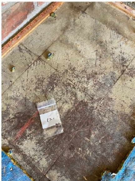
Picture 3: Asbestos-containing brown 9x9 floor tile
