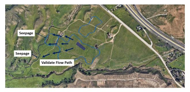
The following illustration shows how it is possible for the recharge water to laterally instead of vertically to the groundwater basin.
