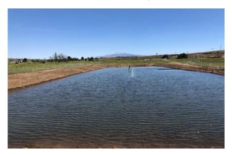
On April 20, 2019, the initial test was stopped to re-evaluate the project due to slow infiltration from the surface to the groundwater. The District staff drained the basin, tested the soils in the basin, and removed additional soil from the basin to reach a more permeable layer of soil. Following the modifications to the basin, the District staff and Geoscience restarted the infiltration investigation.
