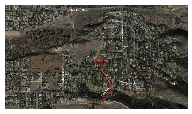
The replacement pipeline consists of 680 linear feet of 8-inch Ductile Iron Pipe (DIP) four drinking water services, two fire hydrants, and one water quality sample station.
