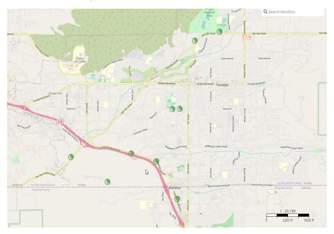
One key element to the District's sanitary sewer monitoring system is the use of flow monitors that actively monitor sewer flows throughout the District. The data collected consists of depth, velocity, and quantity of sewage that flows past a monitoring station. The graph below shows the weekly trends of sewer flow characteristics at Lift Station No. 1.
