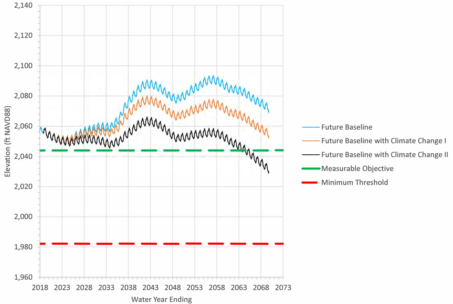
Figure 3-22. Predicted Hydraulic Heads at South Mesa 7 in the Calimesa Management Area
