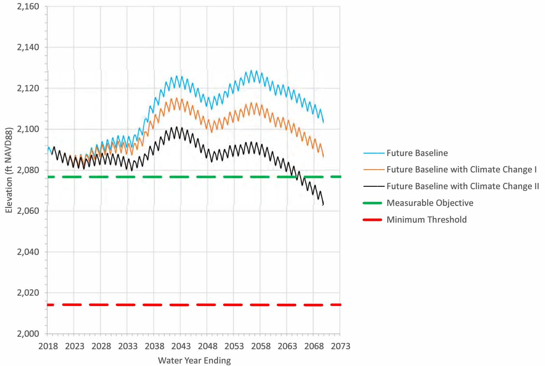
Figure 3-26. Predicted Hydraulic Heads at YVWD-10 in the Calimesa Management Area
