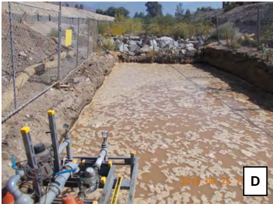
A. YVWD hydrant at 10th Street and 4" fire hose B. 4" fire hose along northern channel bank west of 10th Street C. Excavated basin, fencing, and soil stockpile D. Initial test basin filling (Day 1) E. Falling head test in progress view from south (Day 2)
