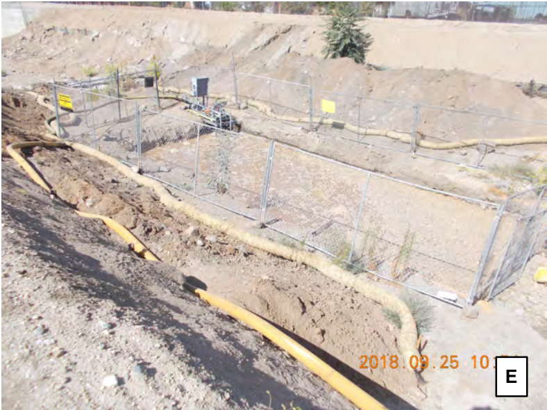
A. YVWD hydrant at 10th Street and 4" fire hose B. 4" fire hose along northern channel bank west of 10th Street C. Excavated basin, fencing, and soil stockpile D. Initial test basin filling (Day 1) E. Falling head test in progress view from south (Day 2)
